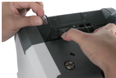
Banknote Guider Uninstallation
