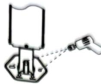
2. According to the size of the base mounting hole, make two mounting holes on the wall.
